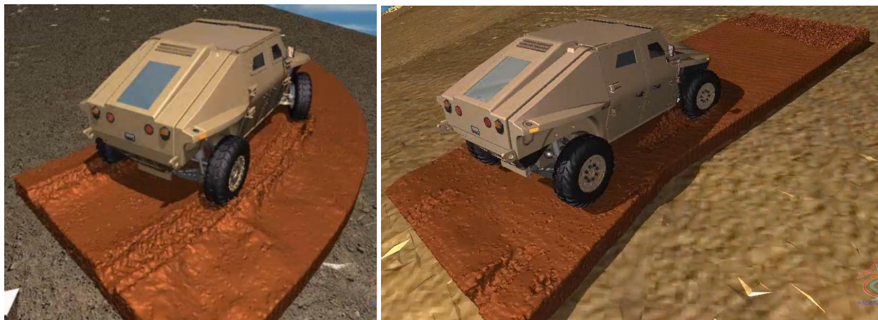
Figure 68: Snapshots of the moving DEM complex topography terrain patch in typical vehicle mobility simulations: 90° turn (left) and going down a slope (right) on rough soft soil terrains.
