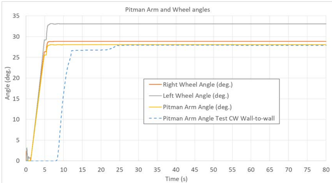
Figure 29: Wall-to-wall turn radius simulation time-histories of pitman arm, inner (left) wheel, and outer (right) wheel angles. The test pitman arm angle is also shown for comparison.
