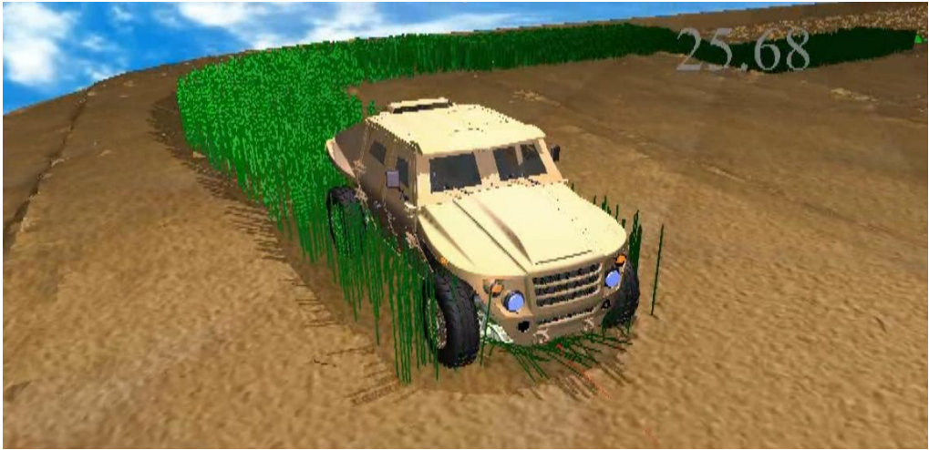
Figure 90: Coupled vegetation – vehicle simulation. Vegetation blades are modeled using thin beam elements.
