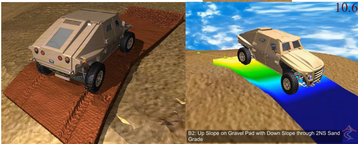
Figure 78: Snapshots of the FED vehicle crossing the B2 (Down Sand Grade with short length of gravel pad) segment.
